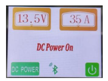
The LCD screen above will be displayed when the user activates DC Power mode by pressing the "DC Power" button, the output voltage and current will be displayed.
