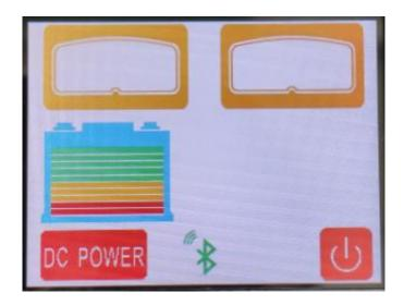
The LCD screen above will be displayed when: the user presses the power button on the bottom right corner of the monitor to turn off output from the charger, the charger still has 240VAC power and is within the wireless range of the LCD monitor. The output voltage and current will not be displayed, but the battery capacity of the connected battery will still be displayed.
