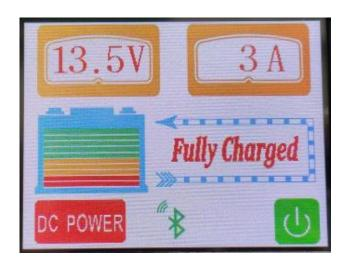
The LCD screen above will be displayed when after the In Progress stage. The "Fully Charged" words will display during the final maintenance stages.
