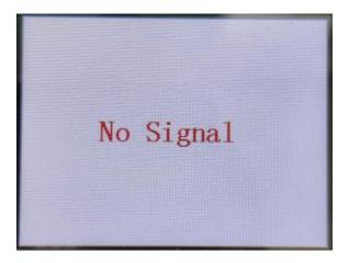
The LCD screen above will be displayed when the LCD monitor is not receiving any Bluetooth signals from the charging unit.
