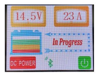
The LCD screen above will be displayed after the Start Charging stage. The "In Progress" words will display during the main charging stages.
